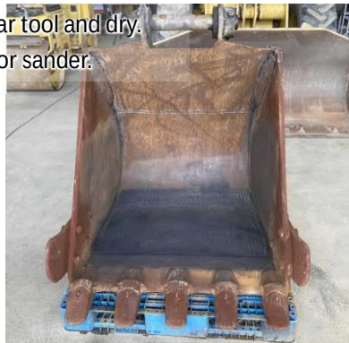
Chipping cleaning completed
